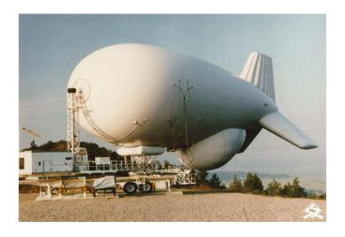
FIG.7 TCOM Land Based Aerostat.
